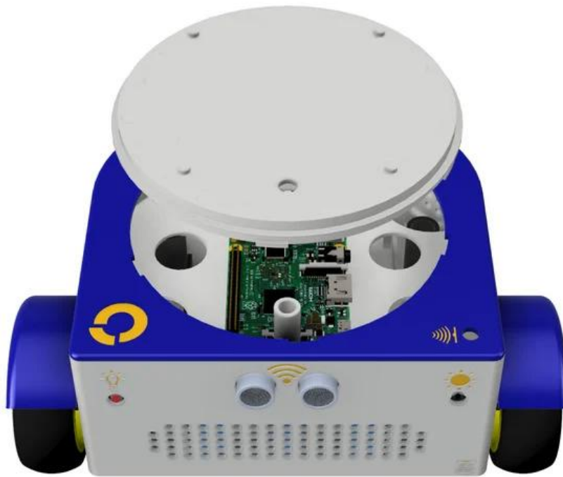
Figure 1. The top-view and internal aspect of FOSSBot's initial design
