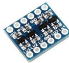
Figure 13. Placement of Bidirectional logic bit converter on PCB
